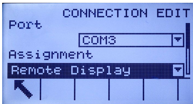
Figure 3-13: COM2/COM3 Connection Configured for Remote Operation
