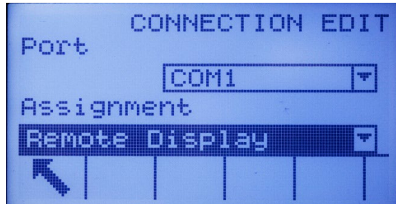
Figure 3-11: COM1 Connection Configured for Remote Operation
