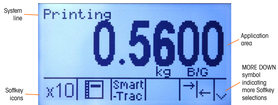
Figure 2-9: Default Home Screen, System Line with Message Showing
