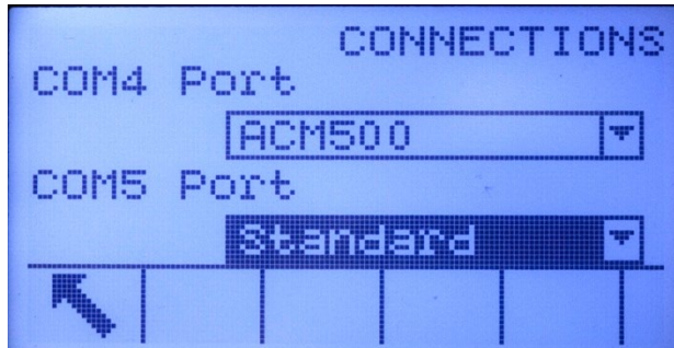
Figure 3-12: COM4 Connection Configured for ACM500
